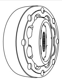
Flip the bearing assembly over and expose the bearings to add grease to this side. Work the grease into the bearings by moving it around.
