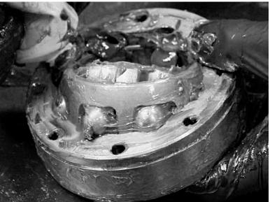
As shown in the picture, grease should surround ALL the bearings and ALL internal parts of the assembly.
