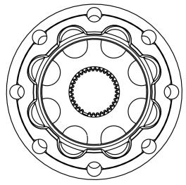
Use the provided grease tube and squirt grease into the bearing assembly. Work the grease into the bearings by moving it around. It will be tight at first, but will loosen as grease is worked into it.
