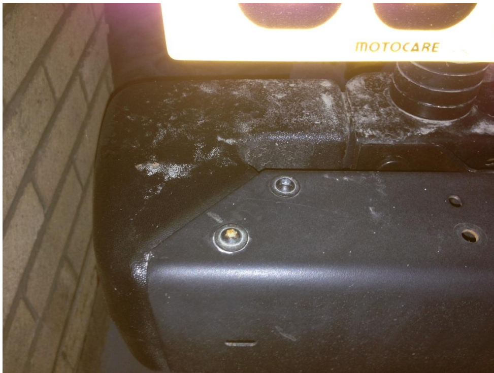
US Spec End Cap (note Bumpers squared off, and bumper still covers up to corner of vehicle)
