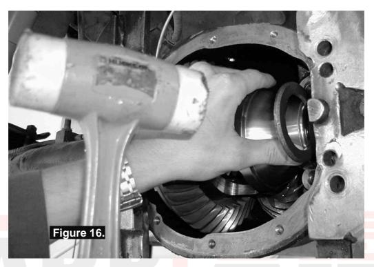
NOTE: If the master shim is too tight to fully install then the spreader tension may need to be increased. Do not
