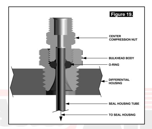
NOTE: Excessive tightening of the center compression nut is not necessary to form a good seal around the tube and may damage the O-ring, the seal housing tube, or the threads of the compression nut.
