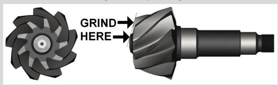
Clean all grinding particles from the pinion gear & differential housing after modifications.
