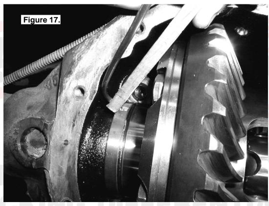
NOTE: The seal housing tube should lay as low in the seal housing groove as possible.
