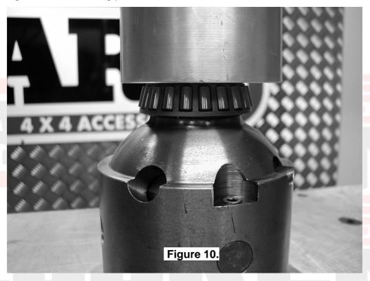
Invert the Air Locker and press the other tapered roller bearing cone onto the opposite bearing journal of the differential carrier until the bearing seats firmly against the bearing journal shoulder.
