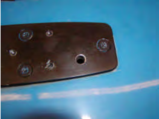
Figure 3. The first hole needs to be drilled in this location through the hinge and outer door.
