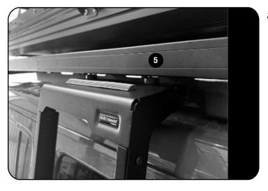
Place the tube spacers (Item 5) over the two top holes on the top mounting bracket and place and fit the top bracket to the bolts inserted in the rack T slots earlier. Place two washers and nyloc nuts to hold in place
