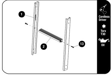
Assemble the Ladder Steps (Item 2) to the Ladder Sides (Item 1) using the M6 x 25 Thread Forming Screws (Item 13).
