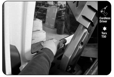
Remove the six M8 bolts holding the Rear of the roof in place using a T50 Torx.
