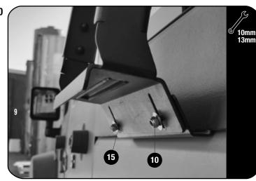
Line up the ladder with the Bottom mounting Bracket.
