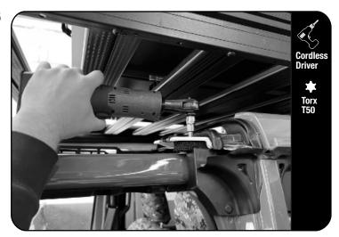
Remove the two M8 bolts holding the front of the roof in place using a T50 Torx.
