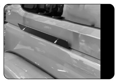
With the help of a friend, Lift the Roof just enough to slip in the Bottom mounting bracket between the Roof and Body.
