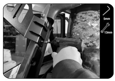
Remove the fasteners securing the internal rack mounts to the rollbar. Four on rear mount and two on mid mount.
