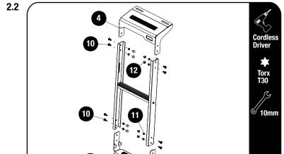
Assembly the Top Mounting Bracket and Bottom Mounting Bracket (Item 3 & 4) to the assembly done in step 2.1 using M6 x 16 Flanged Button Head Bolts (Item 10) and M6 Nyloc Nuts (Item 11) and fully tighten. Place the M6 Nut Caps (Item 12) over the M6 Nyloc Nuts.
