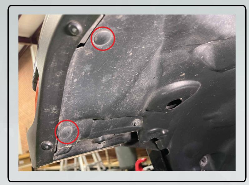
2. Towards the back of the fender, remove this (1) one 10mm bolt, and (2) two push clips.
