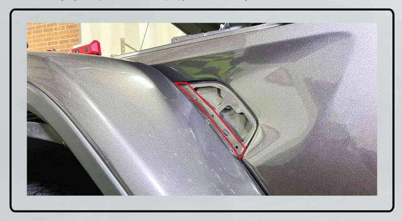
9. Pull back the backing off of the double sided tape. and install the side marker onto the fender.
