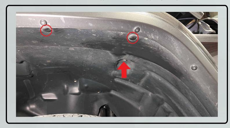
3. Pull the fender liner down and locate this connector toward the middle of the fender. Unplug it by sliding the red tab back, then press the release tab down, and slide the connector apart.
