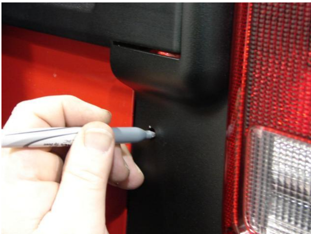
4. Mark the holes and center punch.
