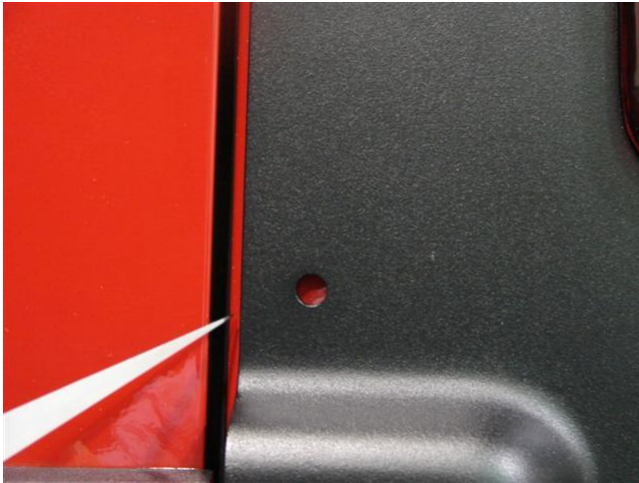
4. Mark the holes and center punch.
