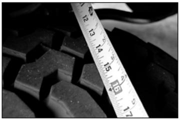
*HINT:* For example, measure from the edge of a tire tread lug to the outboard side of the chassis, then repeat the measurement on the other side of vehicle using exact same points.
