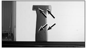
Remove the spare tire mounting bracket from the tailgate by removing the 8 bolts using a 13mm socket.
