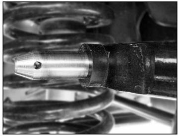
Apply medium strength threadlocker to the tip of mounting post threads.
