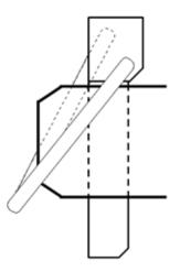
When properly installed, the ring on the Click Pin will "snap" against the shaft of pin. When installed backwards, the ring does not fit snugly against shaft.
