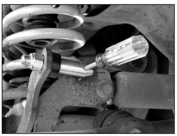
**HINT:** A small Philips head screwdriver or punch inserted into the Click Pin hole will enable you to prevent the mounting post from rotating when tightening the nut.
