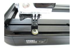
(C) Position as desired and tighten fully, cover the Hex Bolt Head with the M8 Plastic Nut Cap (Item 6).
