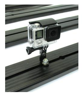
(C) Position as desired and tighten fully, now cover the Nyloc Hex Nut with the Plastic Bolt Cap (Item 6) to finish off the Job.
