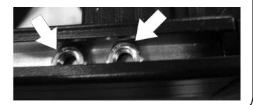
( **B** ) Place one of the Spade Brackets (Item 4) over the outside of the side profile of your rack. Line up the hole in the bottom of the bracket with the hole found between two slats on the bottom lip of the side profile. Secure the Ratchet Buckle (Item 6) and Spade Bracket to the rack using a M8 x30 Button Head Bolt, M8 Flat Washer and M8 Nyloc Nut (Items 2, 4, 7).
