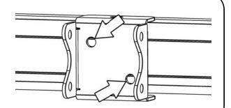
(B) Insert a M8 x 25 Button Head Bolt and M8 Flat Washer (Items 1 &2) through the Ladder Strap (Item 3) and fasten it to the Spade Bracket using a M8 Nyloc Nut (Item 4) as shown.
