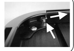
( **D** ) If you have other accessories fitted to your rack, you may need to loosen a bolt or two, allowing you to lift the bolt (nut still attached) to pass the Nyloc Nuts underneath.
