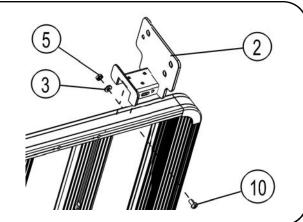
( C ) If you look closely at the Corners of your Rack, there is an opening in the Corner to slide a M8 Nyloc Nut into the "T-slot" Channel of your Rack. Take two M8 Nyloc Nuts and slide them into the channel with the "Dome"side of the Nyloc Nut facing down.
