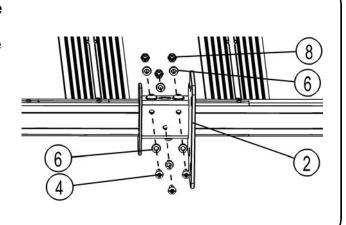
(B) Secure the M12 Machined Pin and Nyloc Nut supplied to the bottom outer hole of the Base Bracket as shown in image using the 17mm Flat or Socket Wrench. Insert a screwdriver or suitable object into the shaft of the Machined Pin through the hole as indicated by the arrow to stop the Pin from rotating while fastening.
