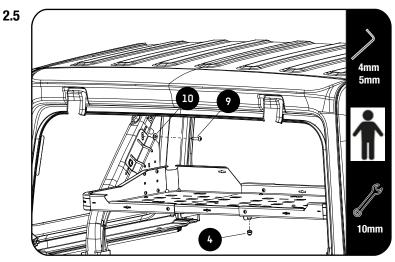
Remove the two plastic covers located on the inside of the roll bar.
