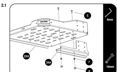
Assemble the Side tray and Side Tray support using M6 x 12 Button Head Bolts and M6 Nyloc Nuts (Items 5 & 7).
