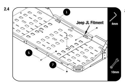
Loosely assemble both Side Trays to the Center Tray (Item 1) using M6 x 12 Button Head Bolts and M6 Nyloc Nuts Items 5 & 7).
