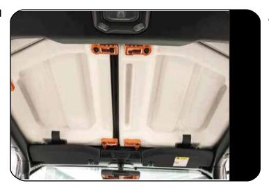
Start by removing both freedom panels from the vehicle.
