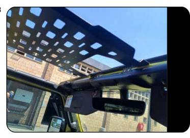
Align the front mounting tabs on the Molle Panel with the OEM mountings of the front catches and loosely refit the front catches together with the Molle Panel using the OEM fasteners removed earlier.
