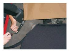
Locate Weather Strip and attach it to tailgate by inserting tailgate into the channel on the Weather Strip.
