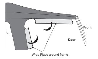
15. Wrap the door flaps around the door surrounds and attach back on the inside of the top with the velcro. Repeat for other side.
