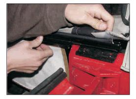
14. Insert the two flaps at the rear window into the rear corner channels on both sides of the tailgate as shown below.
