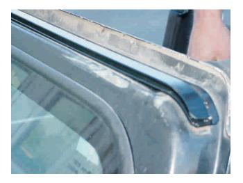
**WARNING:** Ensure Windshield Channel is properly secured prior to installing the Soft Top. Damage to the vehicle or personal injury may occur if Windshield Channel is not securely mounted. Rampage Products is not responsible for personal injury or damage to the vehicle if Windshield Channel is not secured properly.
