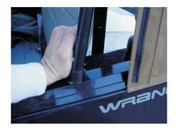
4. Insert rear corners of top into rear Corner Belt Rail.
