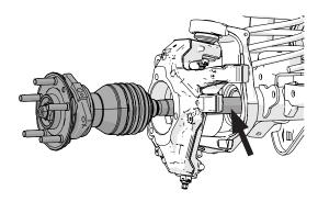
SUPPORT THE INNER AXLE SHAFT SO THAT THE INNER SEAL IS NOT DAMAGED DURING INSTALL.
