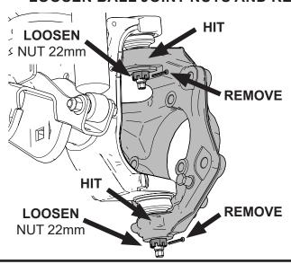
REMOVE COTTER PINS AND LOOSEN UPPER AND LOWER BALL JOINT NUTS BUT DO NOT REMOVE.
