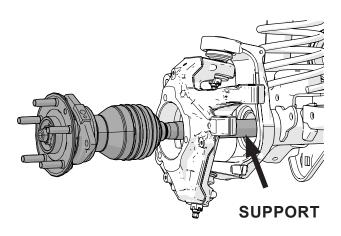
SUPPORT THE INNER AXLE SHAFT SO THAT THE INNER SEAL IS NOT DAMAGED DURING REMOVAL.
