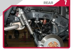
· Install rear shocks with shaft down (Shock #1: passenger side: Shock #2: driver side - ensure reservoirs face rearward)
