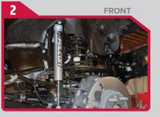
Install Falcon front shocks with shaft down
