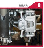
Rotate shaft until lettering on roost • Torque lower bolt to 56 lb-ft
