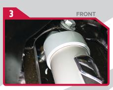
Orient offset eyelet sleeve with spacer facing inward for maximum frame clearance Torque upper bolt to 56 ft-lb
