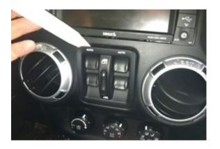
Step 21: Disconnect harness from window switches.
