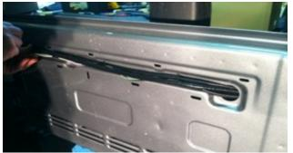
**Step 9:** Use supplied Wire Ties to secure Chassis Harness to fabric factory wire cover. CAUTION: Leave enough slack to allow gate to open fully.
