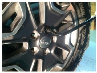
**Step 2:** Slide Camera on studs placing harness end on top of tire carrier. *Do not run harness through the camera bracket opening*.
