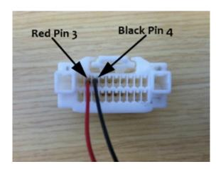
**Step 32:** Connect White 22-pin Connector to radio along with all remaining radio connectors before reinstalling radio head unit and all trim removed.
