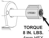
WHEN KNOB BOLT STARTS TO GET TIGHT ALLOW KNOB TO ROTATE TO THE FIRM POSITION AND FINISH TIGHTENING BOLT.
