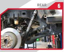
· Install the rear shocks with the shaft down.
