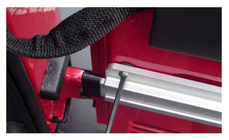
**NOTE**: the rubber lock nuts are designed to compress as they are tightened. This will lock the slider into place.
