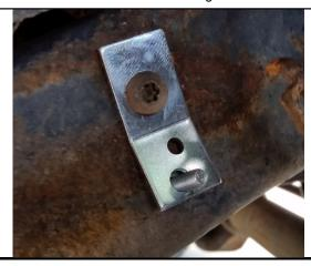
Using the supplied 1/4" nut and bolt, secure the factory bracket to the new bracket.
