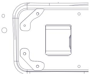
Note location of spacers, place gasket between spacer and tailgate. Apply thread locking compound and install bolts
