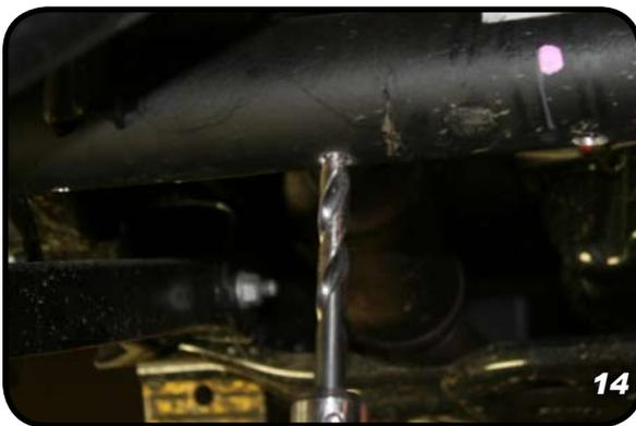
18. After all the holes are drilled blow the metal shavings out of the tubes.
