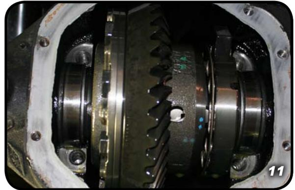
15. Remove the carrier by placing a 19mm wrench on the ring gear bolts and turning the carrier so the wrench wedges at the top of the housing, then use a pry bar on the ring gear to roll out the carrier. Make sure not to mix up the bearing caps or shims. (Photo #12)
