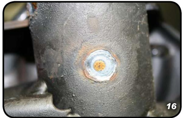
22. To finish welding the sleeve weld the outside of the sleeve where the taper meets the factory tube by the knuckle.
