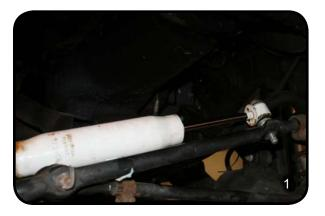
Install the new mounting pin into the steering stabilizer using the new nut and washers supplied and torque to 35 ft-lbs (photo #2)
