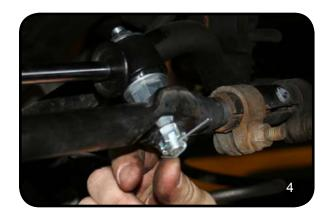
Insert new sleeve bushings into the new steering stabilizer shock, make sure you use ones that fit your factory hardware. If tight, tap them in with a hammer. (Photo #5,6,)
