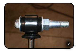
Install the assembly into the drag link, use castle nut and torque to 35 ft-lbs. If alignment is off for cotter pin, back out the castle nut until you can get the cotter pin through the hole on the mounting pin. Use diagonal cutting pliers to bend cotter pin over nut. (Photo #3,4)
