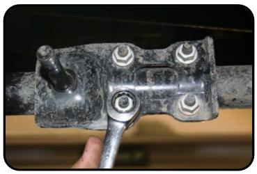
6. For the 2007-2009 JK Wranglers: Some OEM tie rod brackets need additional clearance on the bent flange. You can install the stabilizer and check for clearance or remove the bracket completely and grind the clearance now. To grind the clearance, mark your bracket as shown and remove the small arc of material using a bench grinder or deburring tool. Another option is to replace you tie rod clamp with the 2010-current clamp, Mopar # 68066693AA.
