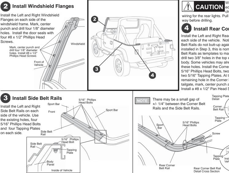
When drilling in the top CAUTION edge of the vehicle body, check underneath for
