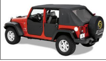
Use of this product will eliminate the factory side mirrors and requires the removal of the entry light bulbs.
