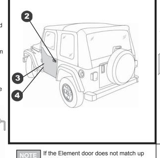
**NOTE** If the Element door does not match up with the door striker, you may adjust the door striker by loosening it with a T-50 torx wrench and either lowering or raising the door striker. Tighten the door striker securely after adjusting. The door striker will have to be put back into it's original position to reinstall O.E. doors
