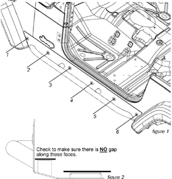
4. Position the guard in place along the body side. From below, begin by positioning the front of the guard, pull away the rear flare from the body side when raising the rear into place. Using a floor jack, press the guard up until the surfaces of the guard touch the bottom of the floor pan as shown in Fig. 2. Centre the guard front to rear.
