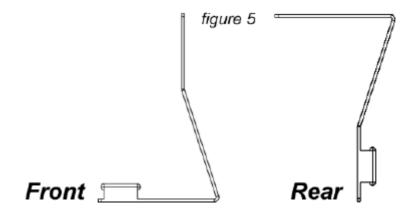
10. Pull the rear fender away slightly and position the assembled cage nut and bracket into the oval hole in the body side; Remove clear tape if present. Using one M6x25 stainless steel button head screw and neoprene washer – insert through hole #6 (Fig. 6) and carefully thread into the cage nut. Tighten until the neoprene is compressed and the bolt is tight.
