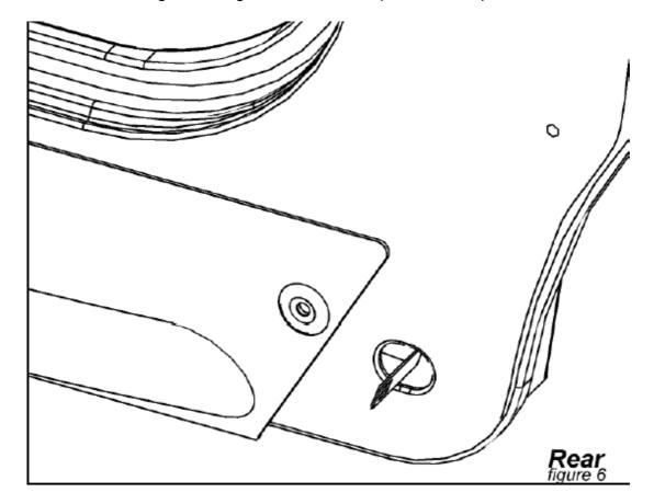
11. Gently push in the part of the cage nut bracket sticking out and fasten rear fender flare down using stock hardware.
