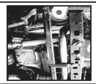
Step 2. With the factory skid plates removed, begin mounting the new transfer case skid plate. Using (3) of the supplied M12 x 35mm hex bolts and M12 washers, fasten the skid plate to the vehicle cross member. Leave these bolts loose at this time.
