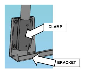
18. Loosely fasten assembly at rear of vehicle as shown using existing hardware removed in step 4.
