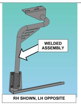
17. Loosely assemble rear mount bracket and welded tube assembly using clamp and M8 hardware supplied in kit.
