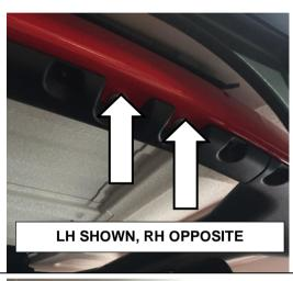
3. Open the rear doors and locate the 2 holes shown within the roll bar on the side of the vehicle above the rear seats.
