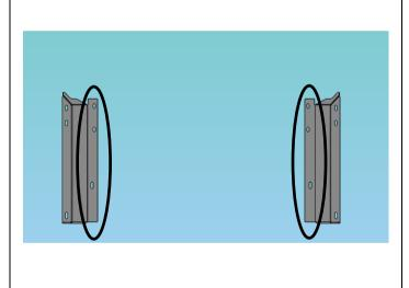
Looking upwards, mark forward 6 centre hole positions onto inside of roof using slots in mount brackets as guides for front mounts.
