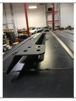
21. Put blades back on and fasten with SS M8x35mm button heads along with m8 nylocks. Make sure to put the button head side on the interior side.
