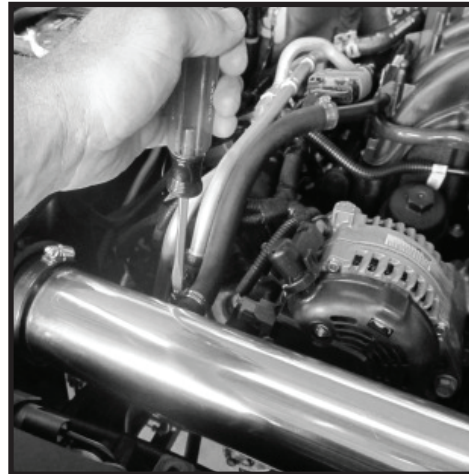
Connect breather hose with clamp
