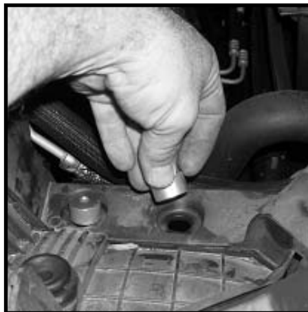
Place spacers on top of tray
