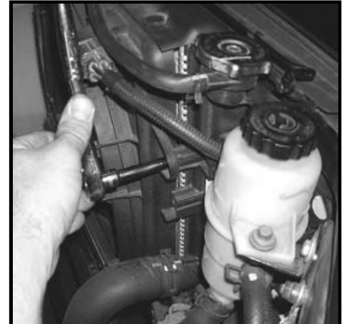
Remove upper shroud bolt
