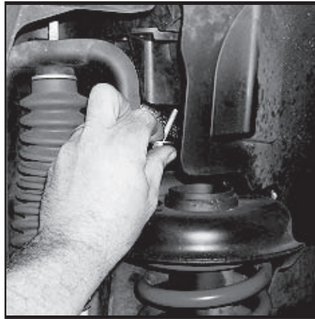
Install bolts from below
