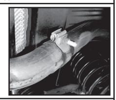
Step 2. Remove the muffler from the (2) rubber isolator mounts. A spray lubricant may be need.
