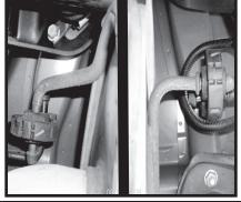
Step 3. Install the new exhaust by first attaching the muffler to the rubber idolator hangers.
