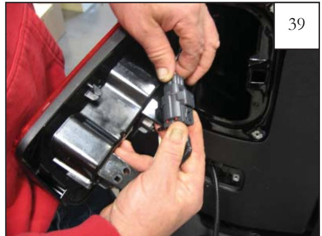
39 Reconnect light connector of tail light.
