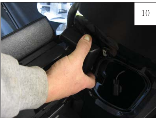
Slide covers off door hinges.
