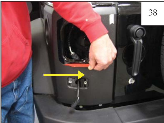
38 Pull tape liner 11 to the right toward the passenger side of the vehicle. NOTE: Refer to step 24 for tape liner tab numbering.
