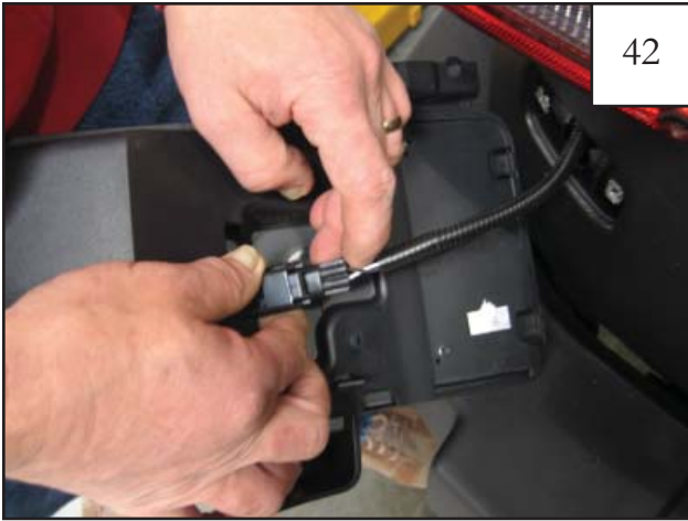
Reconnect light of license plate frame.
