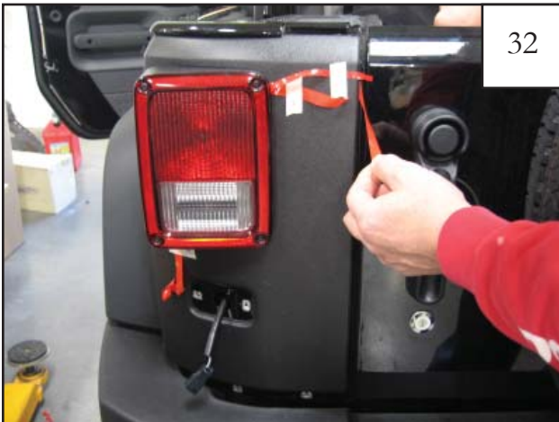
Pull tape liner 7 downward. NOTE: Refer to step 24 for tape liner tab numbering.
