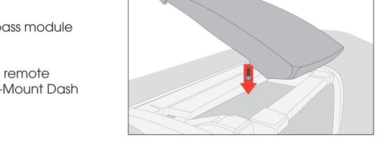
4. Install Multi-Mount Dash Storage by snapping front lip into dash, then pressing back tabs into place.
