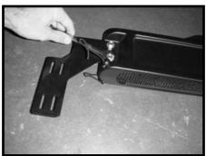
2. Place the Storage Console inside the vehicle such that the mounting brackets rest on the roll bar. The Storage Console should sit just above the visors. Insert Long Velcro Straps through the slots in each Mounting Bracket and strap them tightly around the roll bar on both sides of the vehicle.
