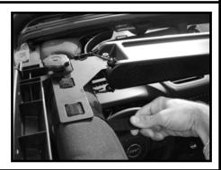
3. Insert the Short Velcro Strap through the slot in the rear of the Storage Console and attach to the footman loop of the windshield.
