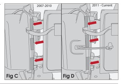
5. Lower rear seats and place Cargo Cover into vehicle as shown. Fabric side will face upward. Loop bungee around rear headrest and secure.
