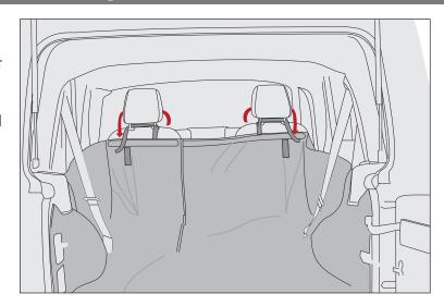
With Cargo Cover secured to front headrests, adjust side door protection cover pieces to side hook and loop strips.
