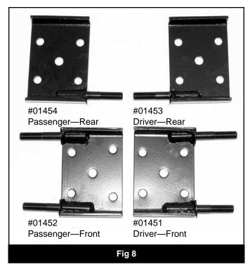
24. Repeat spring removal and installation on the passenger's side of the vehicle. Note: The passenger's side front shackle hanger (#01456) will require installation of (#01493) passenger's side hanger plate spacer and 7/16" x 1-1/2" bolts with 7/16" washers. These spacer plates will provide clearance for the original or certain aftermarket bumpers to be installed. A ½" x 2-1/2 and ½" x 3-1/4" wide u-bolts are required on the passenger's side. (Fig 9)
