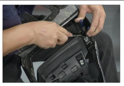
11. Remember to place fender on a soft surface. Now pull the inner fender away from the out fender. These items are glued or fused to each other. Start at the bottom corner of the fender and pry the pieces apart from each other.
