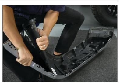
12. The locating tabs need to be trimmed away. A shape box blade works well cutting through the plastic. Feel free to use other tools if you feel fit. Take your time don't rush or force your cut. That could accidently cause you to cut to far or scratch the paint.
