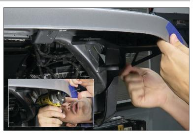
15. We choose to use a step bit to fit the desirable size. You can use standard bits if you prefer. Drill and build up to the size hole needed for the LED light. Test fit the light to assure it fit's snug.
