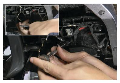
6. Disconnect side marker lights and front running lights. There are some zip ties that will need to be snipped to release the harness from the fender.
