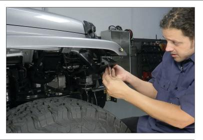
17. Use the provided M6 bolts and washers and attach the bracket to the fender tabs. Adjust and fully tighten.
