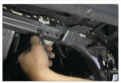
9. Place the fender on a soft surface to assure the paint won't be scratch during modification. First pry and remove all the fender clips to reuse later. Also remove wiring harness from fender.
