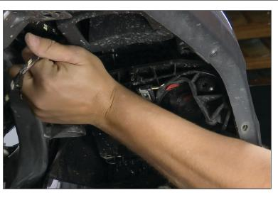
8. Now release all the white retaining clips that attach the fender to the Jeep. Use a small set of needlenose pliers to pinch the back side of the clip and pull the fender from the Jeep. The last clip at the bottom of the fender is deep in the fender. Standard needlenose pliers won't reach it. You could use a long screwdriver or just pull to release this clip. Now fender can be removed.
