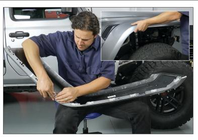
14. Next you need to mark and drill the hole for the side marker light. First apply painters tape to the fender to assist in keeping the paint from being scratched. Now loosely install the Chop Bracket with the 2 fender mounting bolts. Mark the inside of the fender in the center of the hole of the fender bracket. Remove the bracket and drill a pilot hole to the mark you made.
