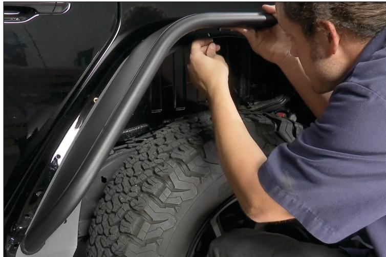
11. Now fully tighten hardware in a alternating pattern. Avoid using power or air tools. The last button head towards the rear of the fender is tight to the tube, it requires a short Allen head key to hold and tighten. This completes the install.
