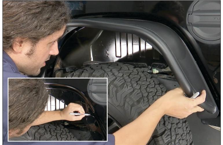
8. There is NO drilling necessary for this install. The nutserts will fit into the factory holes you marked in the previous step. To properly install we highly recommend using a nutsert tool. Insert nutserts into the Jeep body using the tool to crush the nutsert to the body. Take your time and assure each nutsert is crimped fully to avoid it from spinning or from being crooked.
