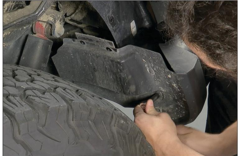
5. Remove the plastic shield from the bumper. It also has three M8 bolts attaching it.
