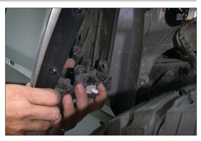
3. Unplug the fender wiring from the chassis harness
