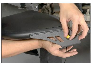
12. Clean the sheet metal of the Jeep where the steel fender will meet. Place fender into place to the vehicle. The brackets will support the weight of the fender.
