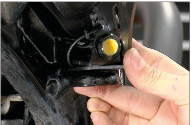
15. Concerning the method of wiring use your preferred method. We selected wire splices with heat shrink ends. We would also recommend soldering and using heat shrink as the best method of connection and keeping the connections waterproof.
