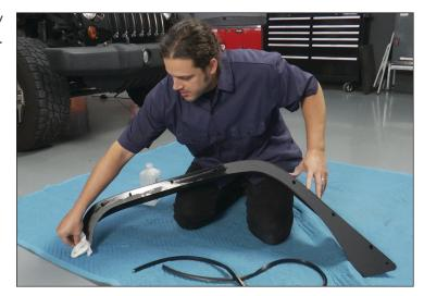
6. When applying the fender seal, peel back a small portion and apply to the fender. Peel and press along the entire top edge of the fender. Once you reach the bottom rear edge of the fender trim seal with a scissors of utility blade.
