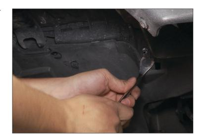
3. Pull the fender away from the body of the Jeep. Pull in a upright and away from the vehicle. Remember to unplug the marker light from the harness.
