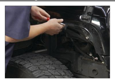
5. To attached the seal to the fender first thoroughly clean the fender surface with degreaser or alcohol. Allow the surface to fully dry before installing the adhesive back seal.
