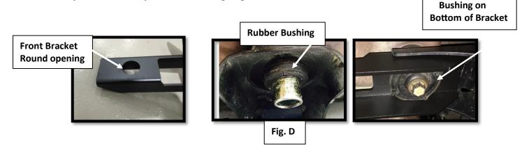
**<u>Step 5</u>**: Tighten all hardware to factory specs starting with the center bracket then front and rear.
