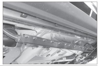
2. Remove rubber plug filling oval hole in bottom of rocker panel in front of two front holes in pinch weld.
