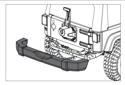
2. Install Left and Right Mounting Brackets into frame rails using Hex Head M12 Bolt, Lock Washer, and Oversized Washer. Do not fully tighten hardware.
