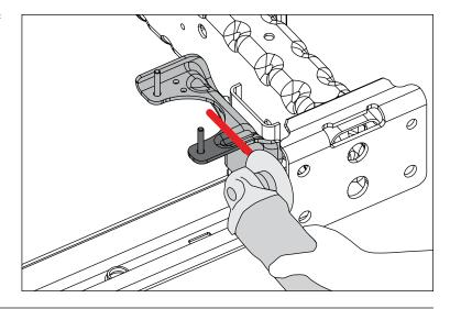
8. Drill a 5/16" hole through cut vacuum pump mounting bracket 1/2" from cut edge.
