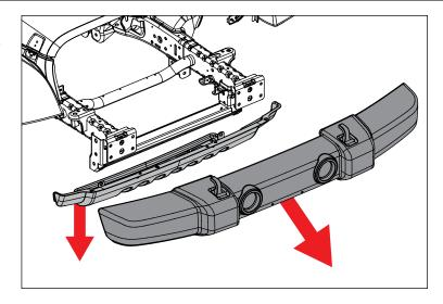
5. Remove factory closeout panel by releasing plastic fasteners along frame rails.
