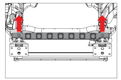
6. Unbolt factory vacuum pump and set aside.
