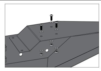
14. Loosely install Spartan Front Bumper and D-Shackle Tabs using supplied M12 hardware. M12 Nut Plates are designed for mounting behind Winch Plate.
