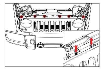
3. Pull bottom of grille away from vehicle to disengage metal clips on bottom rear of grille.
