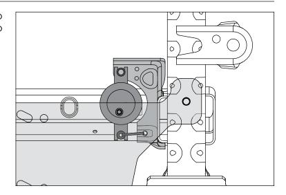
12. Remove fog lights from factory bumper and install on Spartan Front Bumper using supplied M4 hardware.
