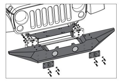
15. Fasten Spartan Front Bumper to Winch Plate using supplied M8 hardware. Tighten all fasteners and reconnect fog lights.
