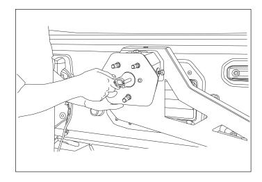
17. Slide the mount to the desired position according to the spare backspacing. This requires measuring the spare to determine the best position. Once in a position is determined, fully tighten all three bolts.
