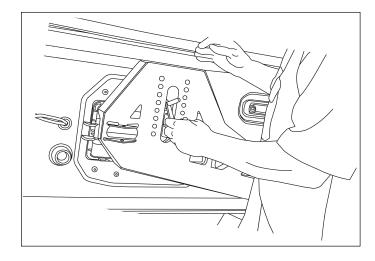
14. Install the tire mount base over the M12 studs to the carrier using flat washers and Nylock nuts. Tighten fully.
