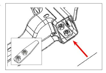
6. It's recommended to place painter's tape to the lower corners of the body to avoid damage to the paint during installation. With assistance, lift and place the bumper to the frame rails. Thread M14 bolt and washer into the side of the frame rails.
