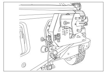
21. Reinstall the passenger side taillight. Requires the same procedure as step 10 in reverse. DO NOT overtighten plastic hardware, avoid damage to these plastic components.
