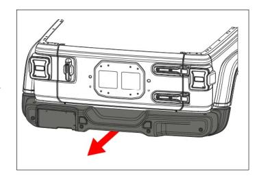
2. Using T25 Torx drive, remove two screws securing the lug stud assembly to the factory tire carrier. Remove the lug stud assembly, including backup camera, and set aside for later use.
